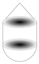
We want composite tank 1 to be at a height 2R to be consistent with the other tanks and so we let H = (2/3)R for each individual tank that makes up our composite tank to achieve our desired height. Note that we will have to adjust the hemisphere's height by multiplying the volume and area by  $\frac{2}{3}$ .
