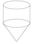
Composite tank 3 is constructed with a cone making up the bottom half and cylinder making up the top half. Admittedly, composite tank 3 does not seem common as the others, however, it should be considered as the cone has the best emptying efficiency of all the conic-shaped tanks. By construction, f(h) = R,  $0 \le h \le \frac{1}{2}H$  and  $f(h) = \gamma h$ ,  $\frac{1}{2}H < h \le H$  where  $\gamma = H/R$ . Hence, we obtain the cross-sectional area
